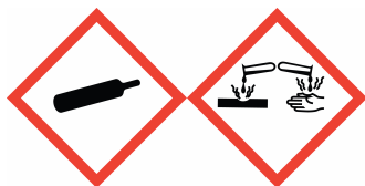
Compressed Gas Corrosive
